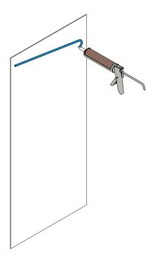
2. On the back of the panel, starting at the top corner, apply a bead of adhesive that is approximatly 1/4" wide.
