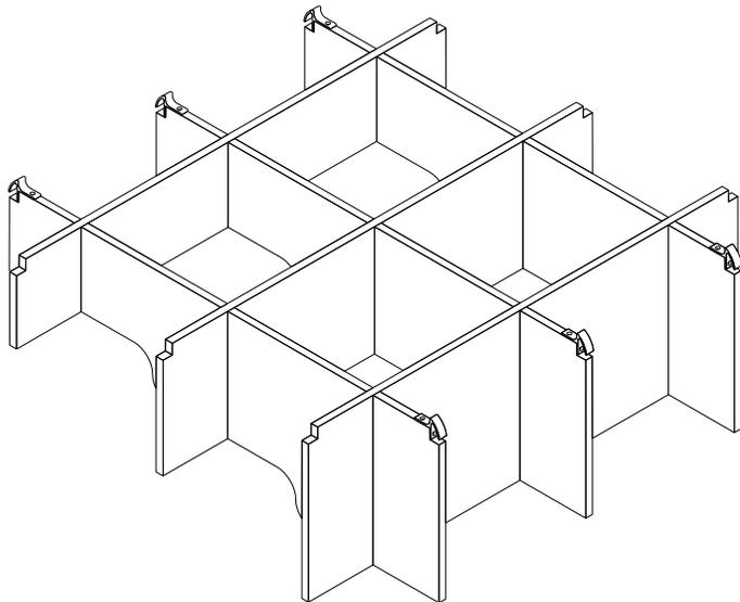
4. Align the tile with the underside of your T-Grid system, then push the tile into the grid to engage the plastic clips. Your tile is now installed.
