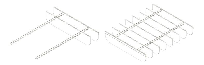
5. Next, attach the 'Clevis-Hook' onto the T-track in the pre-drilled holes.
