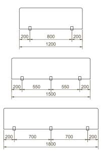
2. Using the dimension diagram shown above as a reference, fix the first clamp section to the desk surface using two screws suitable for your desk material type and thickness...
