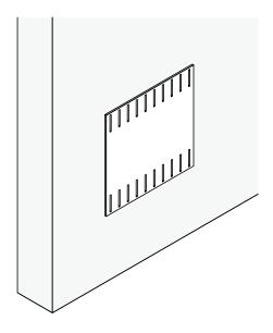
On the back-panel tile, starting at the top corner, apply a bead of adhesive that is approximately 1/4" wide. Continue the bead of adhesive across the tile working in a zigzag pattern.
