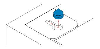
4. Now, holding the panel upright in the desired install location, push the panel firmly against the wall, making sure to only push at the mounting brackets locations. This will cause the EZmark plugs to make small markings on the wall at each bracket location.
